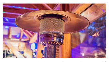
lated area, and not used for extended periods of time, due to the release and potential buildup of lethal combustion products, such as carbon monoxide and nitrogen dioxide. Propane heaters do not require electricity to operate.
